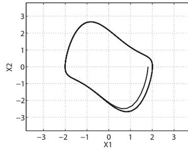
Figure 5: State Response of the Closed Loop with the Initial Condition near the Limit Cycle.
