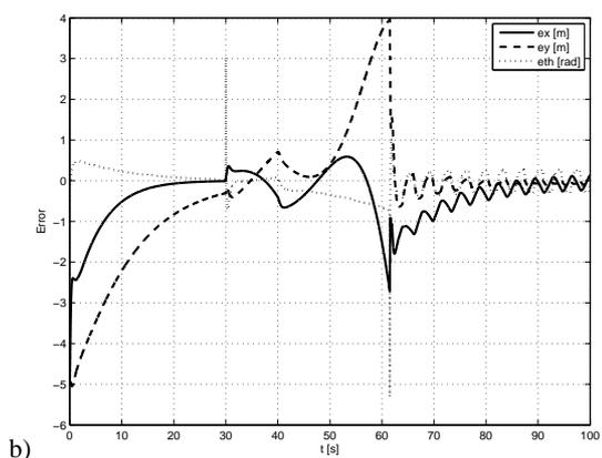
Figure 6: Errors obtained by trajectory tracking with disturbances: a) joint errors in manipulator, b) platform errors.
