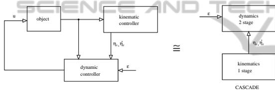
Figure 2: Structure of the control algorithm (backstepping): cascade with two stages.
