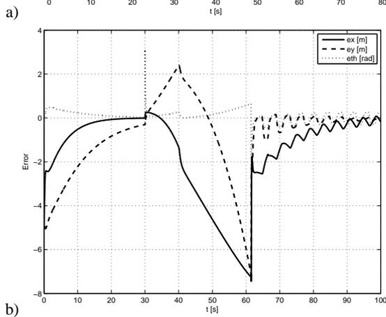
Figure 4: Errors obtained by trajectory tracking without disturbances: a) joint errors in manipulator, b) platform errors.
