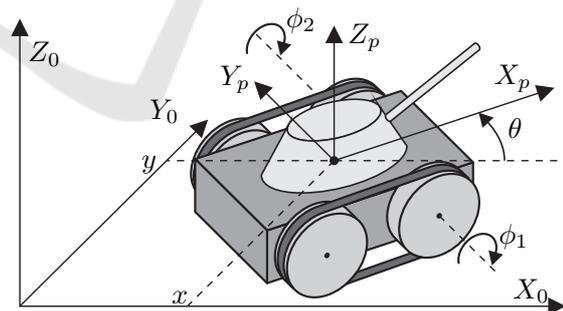
Figure 1: Scheme of mobile manipulator with skid-steering platform – tank with tracks.
