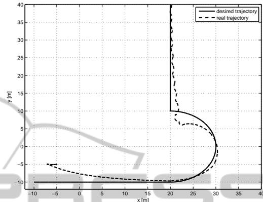
Figure 5: Trajectory realized by skid-steering platform with disturbances.
