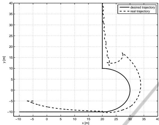
Figure 3: Trajectory realized by skid-steering platform without disturbances.
