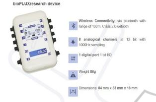
Figure 1: The look and characteristics of the instrument.
