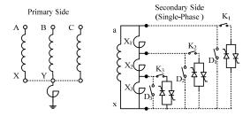
Figure 2: Structure Principle of the 750kV CSR.
