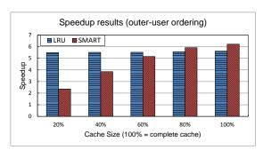
Figure 4: Speedup results for the LRU and SMART caching approaches towards the no-caching baseline for different cache sizes.
