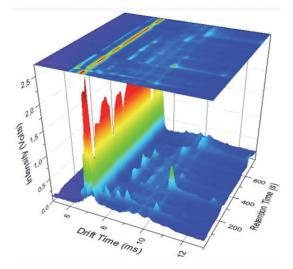
Figure 2: Typical MCC-IMS chromatogram showing characteristic signals of biological matrix.
