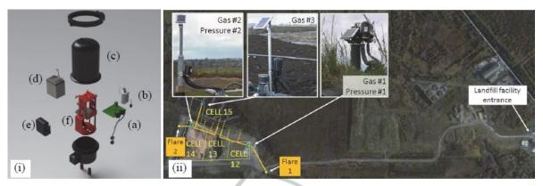
Figure 1: (i) Exploded view of platform (a) microcontroller (MSP430), (b) sensors, (c) IP68 casing, (d) battery, (e) GSM module, (f) extraction pump. (ii) Configuration of wireless sensor network deployed on landfill site.
