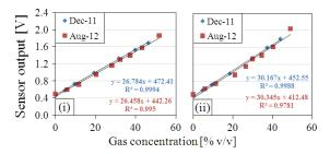
Figure 3: Comparison of sensors' calibration data before and after 8 months deployed (i) CO<sub>2</sub>, (ii) CH<sub>4</sub>.
