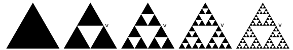
Figure 4: Simplified 2D versions of the Sierpinski shape, embedded in the Euclidean space \mathbb{E}^2 . In this shape, any non-manifold vertex v is shared by two triangles (in black).
