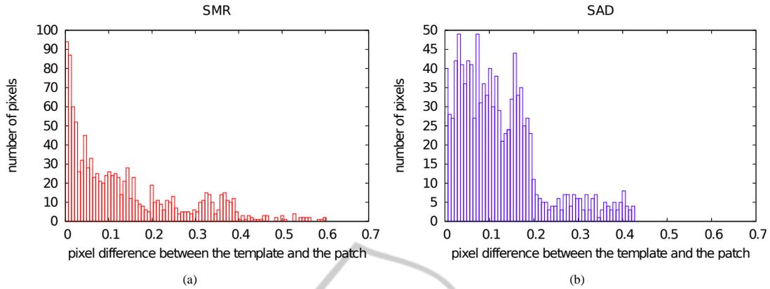
Figure 2: Histogram of the pixel differences that were mapped in Figure 1. (a) Map between the template and result from the SMR tracker and (b) result from the SAD tracker. The SAD tracker minimizes the number pixels with large differences, whereas the SMR tracker maximizes the number of pixels that have small differences.
