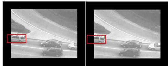
Figure 3: The red boxes are the SMR tracker's outputs. The video frame is extended and padded by zeroes. The SMR tracker is able to track when the target is going out of the frame. The template update is ceased in these situations which prevents the drifting from the object.
