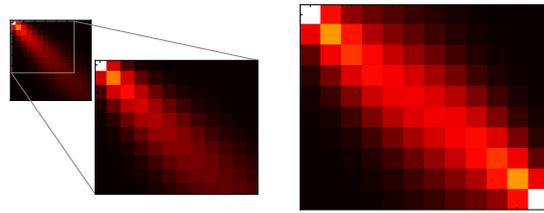
Figure 2: On the left, a precomputed  $15 \times 15$  weight matrix with  $C_{HV} = .3$  and  $C_D = .34$  is used to select a  $10 \times 12$  weight matrix which can then be used to evaluate  $k_{PATH}(s,t)$  for input sizes  $|s| = 10$  and  $|t| = 12$ . On the right, the inversion invariant  $\tilde{\omega}_{PATH}$  corresponding to  $k_{PATH}$  for the same input sizes is displayed.
