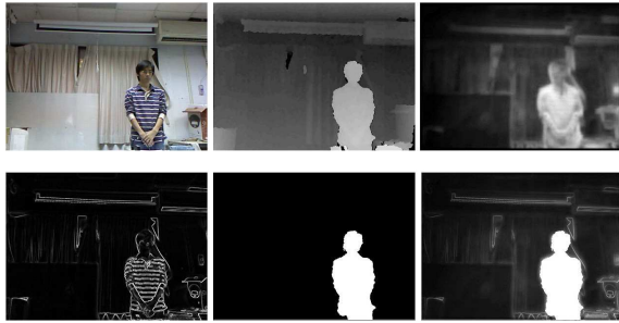
Figure 9: Original image, depth map, saliency map, gradient map, saliency object, and importance map from left to right and top to bottom, respectively.
