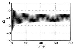
Figure 6: Stablized behavior by cubic state feedback, corresponding to the response shown in Figure 4.
