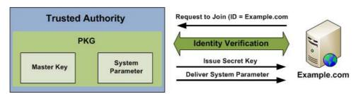
Figure 1: The process of domain joining iSATS.
