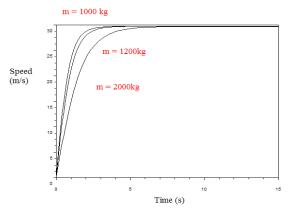
Figure 7: Speed vs. Time with Different Masses (generated by Scilab).
