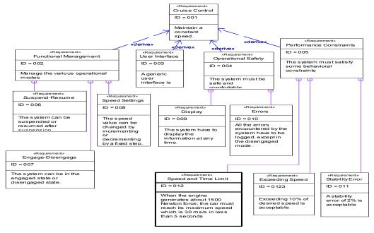
Figure 1: Requirement Diagram of a Cruise Control.
