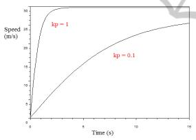
Figure 6: Speed vs. Time with Different Proportional Gains (generated by Scilab).
