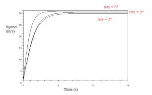
Figure 8: Speed vs. Time with Different Road Slopes (generated by Scilab).
