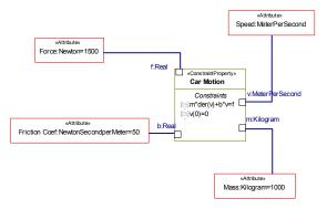
Figure 2: Parametric Diagram of an Open Loop Cruise Control.
