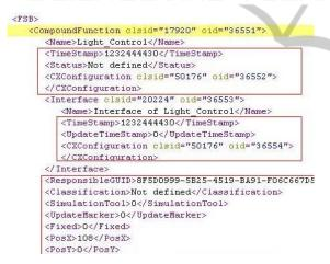
Figure 3: XML Nodes that are not significant for variability.
