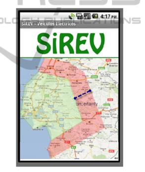
Figure 7: Range estimation based on the uncertainty factors shown in Figure 4.
