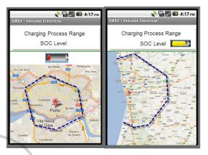
Figure 6: Representation of the charging range for different SOC levels, with a charging process performed in a public charging station in the centre of Porto city. On left, with a low SOC level, a small area is achieved. On right, with almost 90% of SOC level, a large area is achieved.
