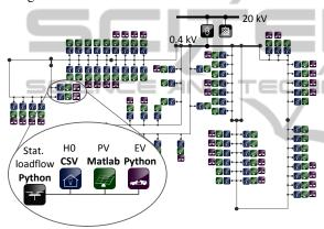
Figure 7: Topology of the simulated rural LV grid.
