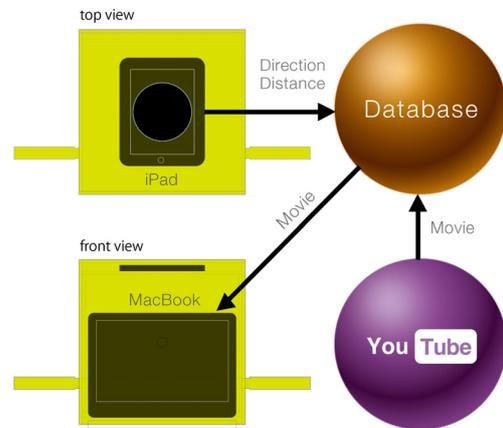
Figure 4: The system configuration diagram.
