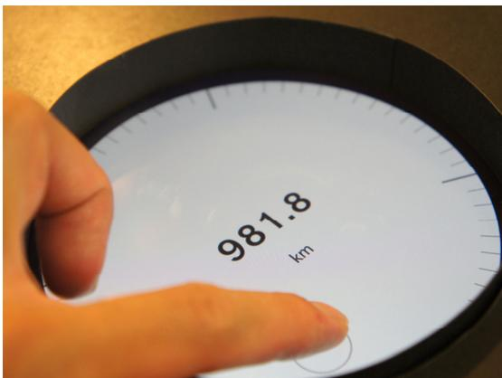
Figure 2: The dial for setting distance.
