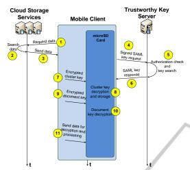
Figure 4: Communication process sequence of  $Sec^2$  key concept.
