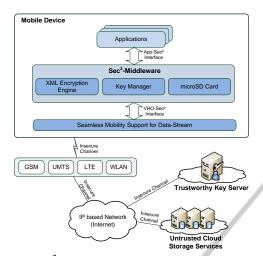
Figure 2:  $Sec^2$  application scenario is based on three parties: Trustworthy Key Server, Untrusted Cloud Storage Services, and a mobile device. The encryption processing and key management within the mobile device is handled by the so called  $Sec^2$  Middleware.
