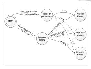
Figure 3: FSM for agents' group formation behavior according to the team captain messages or observations. d<sub>i</sub>: i<sup>th</sup> lowest Euclidean distance between the ball and the agents in the viewpoint, d: Euclidean distance between the agent and the ball, k: the maximum number of attackers.
