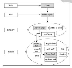
Figure 2: The decomposition of an example plan for an agent that has the *forward* role. Lower level components are hierarchically activated by selection at a higher level. At the lowest level, primitive actions are selected and the corresponding motion commands are sent to the server.
