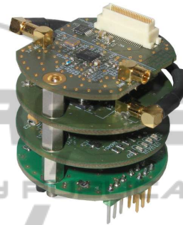
Figure 5: IQlevel mote with battery power supply, MCU, 868MHz transceiver and amplifier module.
