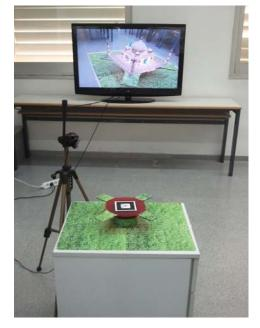
Figure 1: Table with the marker on the rotator support, camera and autostereoscopic display.
