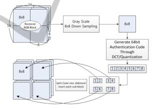
Figure 2: Authentication code generation and splitting.
