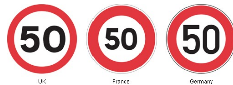
Figure 5: Different countries use different traffic sign design. A detection method that has been trained on UK signs might not recognize French or German signs appropriately.
