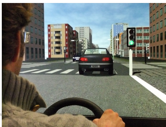
Figure 9: TrafficSimulation used for driving experiments. In this tabletop simulator, a Logitech G27 steering wheel is used as input device, and a 46" sony TV screen, which provides 70 degree of visual field.
