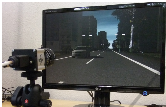
Figure 8: Monitor HIL. The picture shows a scene generated by the simulator under real time conditions. In this scenario, the video data recorded by a CMOS Camera are processed on a standard PC in order to detect lane markings and traffic signs. For analyzing the performance of the detection modules, the ground truth data are also sent via ethernet to the PC. A black box that shields the setup from scattered light has been removed in order to take the photo. See also the video on www.cstlab.net .
