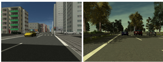
Figure 4: Different scenes created by the Environment Plug-In. A rather rural and a rather urban atmosphere can be achieved by adjusting parameters in the plug-in's configuration.
