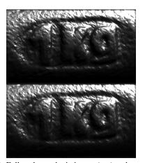
Figure 7: Full-scale synthetic image (top) and corresponding reflectance map (bottom) of the reconstructed surface. The SSIM amounts to 0.985, thus indicating a very high similarity.
