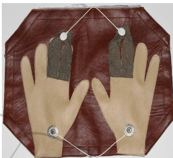
Figure 2: Experimental apparatus: at the top, Electrolycras enable the acquisition of ECG using the index and middle fingers; at the bottom, dry Ag/AgCl electrodes acquire ECG at the hand palms.
