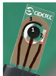
Figure 1: A screen-printed three-electrode system. (1) working electrode; (2) reference electrode; (3) counter-electrode.
