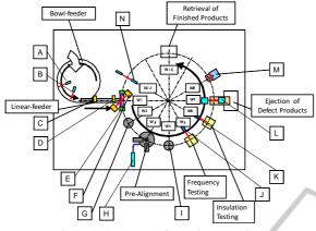
Figure 2: Structure of a testing machine.
