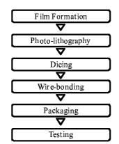
Figure 1: Six major stages of SAW manufacturing processes.
