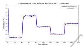
Figure 7: Control evolution with adaptive FLC algorithm for various set points.
