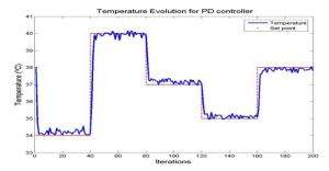
Figure 3: Control evolution with PD algorithm for various set points.
