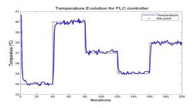
Figure 6: Control evolution with FLC algorithm for various set points.
