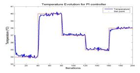
Figure 4: Control evolution with PI algorithm for various set points.
