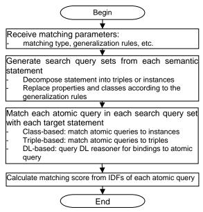
Figure 1: Flow diagram of the semantic matching algorithm.
