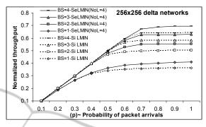
Figure 3: *Normalized throughputs* vs. *probability of packet arrivals* for an 8-stage delta SiLMINs and SeLMINs with 4 layers.
