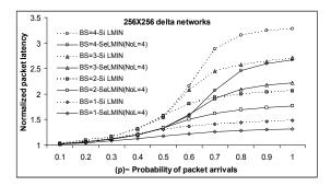
Figure 4: *Normalized packet latency* vs. *probability of packet arrivals* for 8-stage delta type SiLMINs and SeLMINs with 4 layers.
