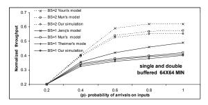
Figure 5: *Normalized throughput* of a 64x64 MIN vs. the *probability of packets arrivals* for b=1 and 2 from various models.
