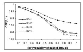
Figure 6: *CPF* of an 8 stage semi-layer delta MIN vs. *probability of packets arrivals.*
