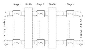
Figure 1: The general structure of a delta network.
