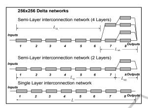
Figure 2: Literal views of 8 layer delta networks (SiLMIN, and SeLMINs).
