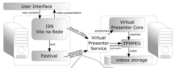
Figure 2: Virtual Presenter architecture integrated to the Vila na Rede ISN.
