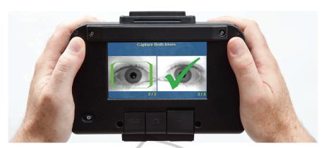
Figure 1: The military mobile iris based identification system HIIDE 5.
