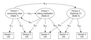
Figure 1: Example of a HMM modeling the activities of multiple people in a smart space. The activities of multiple people are represented as hidden states (circles) and sensor values are represented as observations. The edge labeled with  $a_{ij}$  is the transition probability from hidden state *i* to hidden state *j*, while the edge labeled with  $b_{ij}$  is emission probability of generating observation *j* in hidden state *i*.
