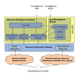
Figure 2: The C@H system architecture.
