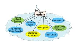
Figure 1: Resource aggregation from many Cloud Providers.
