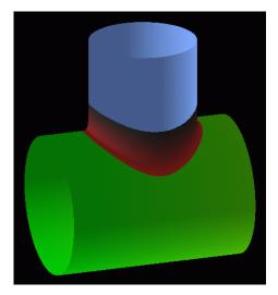
Figure 4: Blending between two intersecting cylinders.
