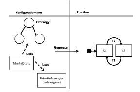
Figure 4: Transition between configuration time (left) and runtime (right) of the HIM manager. The MentalState with the Ontology, and the PriorityManager with the rule engine are transformed into a Cartesian product of machine states, containing all possible inferences. Next, through process of optimization an FSM is created with the minimum number of states.
