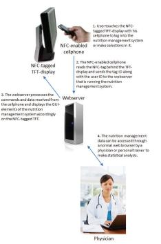
Figure 1: Interaction Process of the TnD prototype system.
