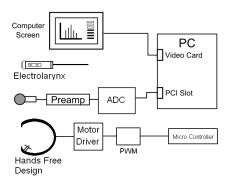
Figure 5: Block diagram of test set up.
