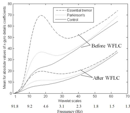
Figure 10: x-gyroscope wavelet spectral analysis for rotational tremor.
