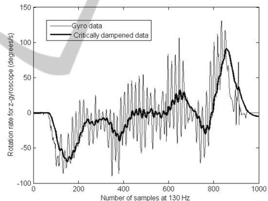
Figure 6: A processed z-gyroscope signal before and after a critically damped filter is applied to approximate *intended rotational motion*.
