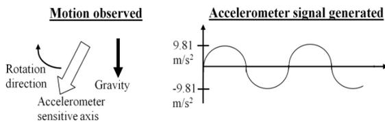
Figure 1: An accelerometer rotated through the gravity field and the signal generated.
