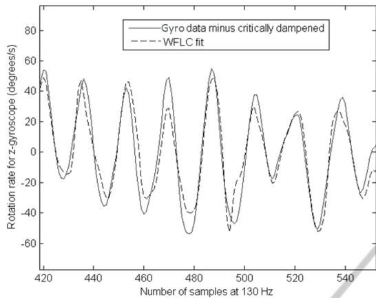
Figure 7: A processed z-gyroscope signal portion and its WFLC approximation depicting rotational motion.
