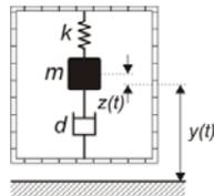
Figure 3: Basic mechanical representation of an inertial generator.
