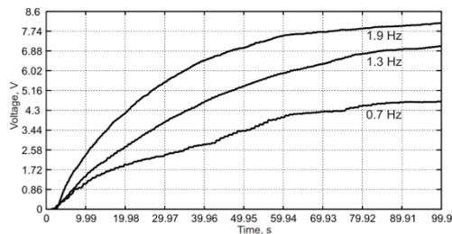
Figure 9: Capacitors' voltage evolution over time.
