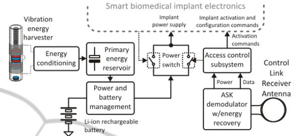
Figure 2: System overview with special focus on the energy harvester and system activation modules.
