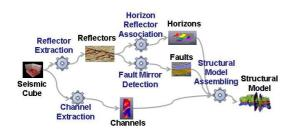
Figure 1: Simplified fragment of a potential seismic interpretation workflow.
