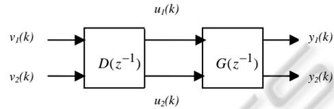
Figure 1: The structure of the decoupled process.
