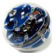
Figure 2: The standard ball with IR Sensors.
