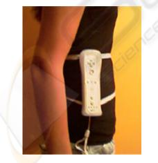
Figure 3: Correct placement of the sensor in the trunk.
