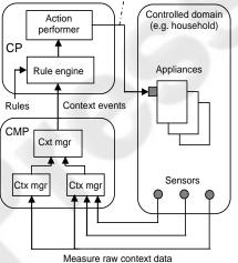
Figure 3: ECA pattern applied to home nergy management (CP = Control Process, CMP = Context Management Process.
