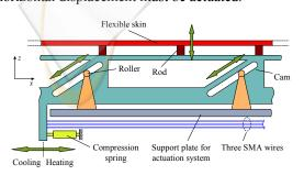
Figure 1: The actuation mechanism concept.
