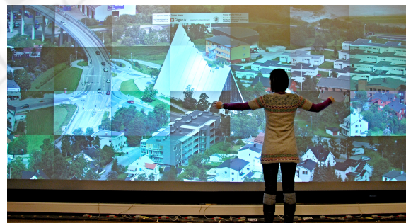
Figure 1: A user navigates in a 13.3 gigapixel image on a 22 megapixel tiled display wall using hand- and arm-gestures.
