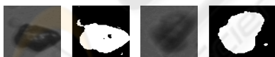
Figure 7: Some crystal like particles are shown in the figure. In spite of the relative low difference between background and object and the fact that the samples are semi transparent, the segmentation is good. Even small ones are handled together with the large ones.
