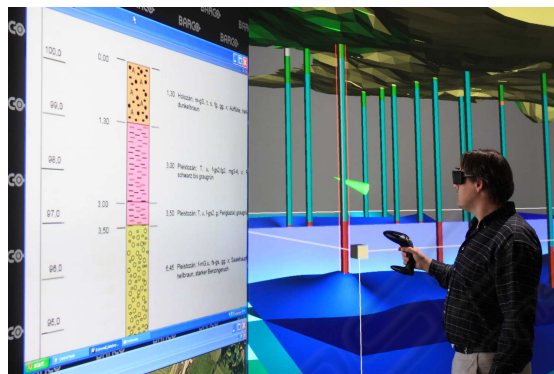
Figure 5: Example of requesting additional information on one of the objects shown in 3D space. The person picks one of the boreholes in order to see the additional 2D information, which is shown on the left screen.
